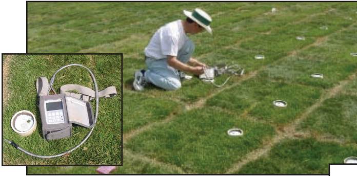
The Field Chlorophyll Fluorometer was developed by Dr. Zhang to perform the Photo Chemical Efficiency Test.
